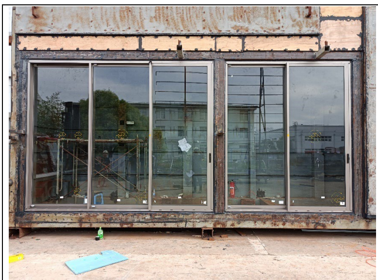
Photo No.4 Specimens #05 and #06 Before impact test (Testing on May 19, 2024)
